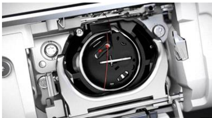
Figure 2. Vertical rotary hook. ( Bernina 770 sewing machine)
